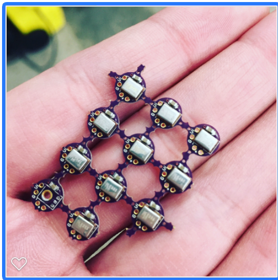
Fig. 1: 6.35mm diameter PCBs with mounted MEMS
